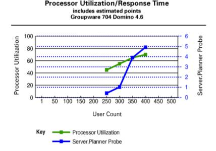
The graph above represents, for system 704, a combination of the amount of the processor used evaluation and the probe response time evaluation.
