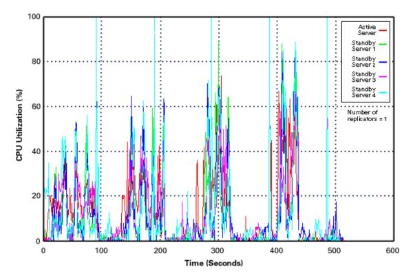
This next chart shows the results with four Cluster Replicators on the active server. Notice that in this chart, the bands are narrower than in the previous one, indicating that the replication occurred faster.
